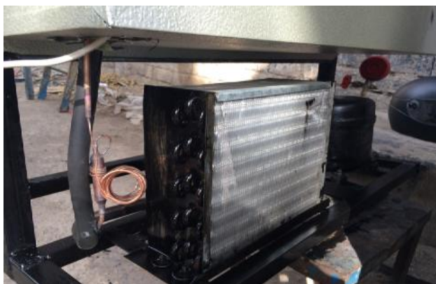
FIGURE 5. CONDENSER AND COMPRESSOR
