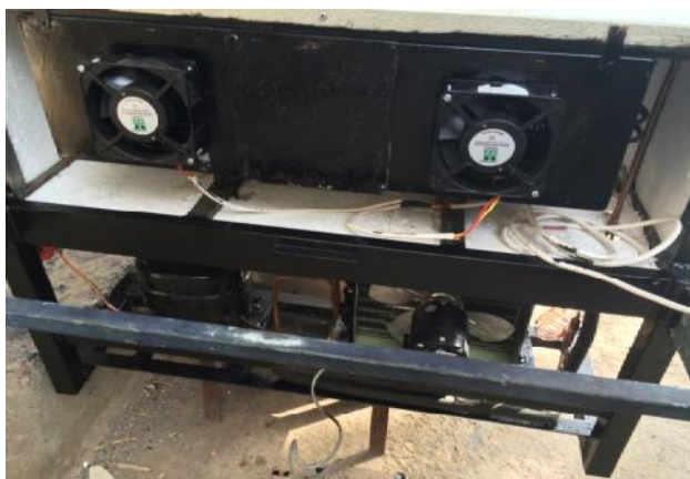
FIGURE 4. COOLING COILS AND EVAPORATOR FANS IS LOCATED IN THE BED HEAD
