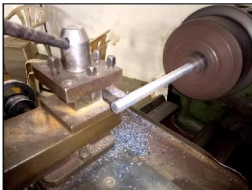
Figure 7 turning the shaft
