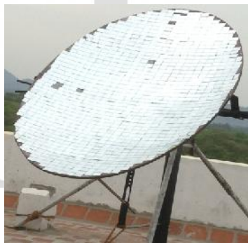
Fig.4 Manufactured 2 m 2 solar Scheffler reflectors at VIT University, Vellore
